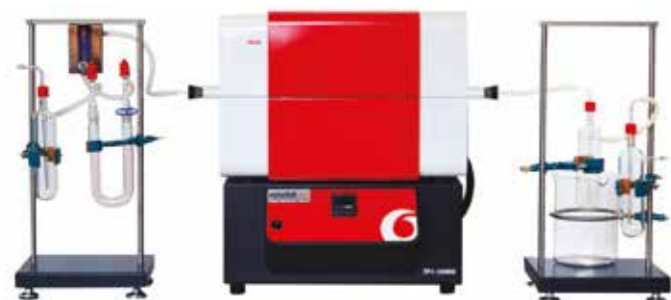
External dimensions of furnace only: 500x340x570 h mm Heated tube length: 400 mm ± 5°C temperature uniformity in 196 mm length Weight: 37 kg
