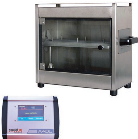
Dimensioni/Dimensions: 285x204x360 h mm Peso/Weight: 13 Kg Gas: Metano /Methane Propano/Propane
